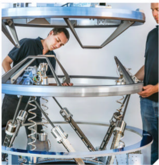
Engineers inspecting a pre-production prototype of the IBDM
