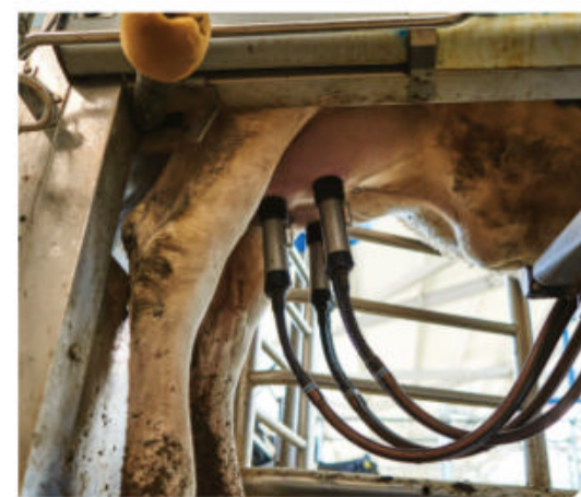
A robotic arm automatically attaches the milking cups when the cow steps in
