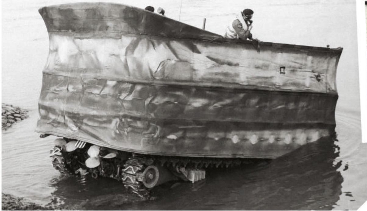
One of Hobart's swimming Duplex Drive tanks entering the water
