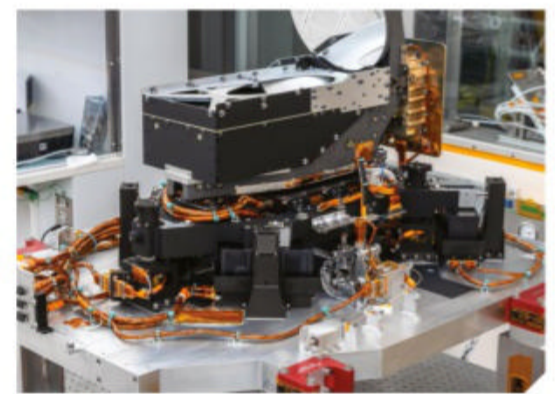
The Deep Space Optical Communications (DSOC) experiment on board Psyche
