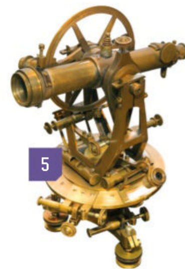
As the surveyor rotates a theodolite towards the new focus point, the angle between the distant locations is measured
