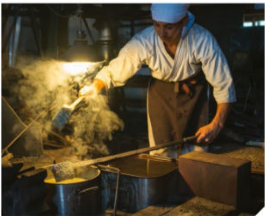
A Japanese swordsmith covering a blade in a layer of hot steel slurry
