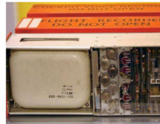
FDRs are able to survive temperatures over 1,000 degrees Celsius
