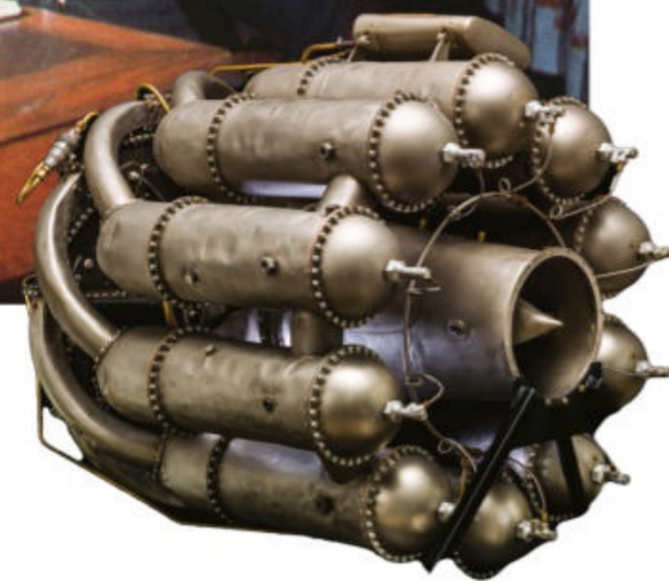
Whittle's Power Jets W.1 engine, used in the Gloster E.28/39 and as the basis for the Rolls-Royce Welland and General Electric's J-series engines
