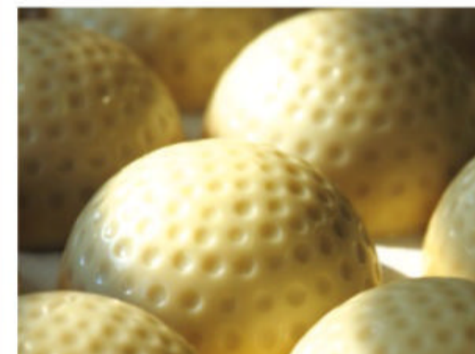
Golf ball dimples are created by filling moulds with plastic around rubber cores
