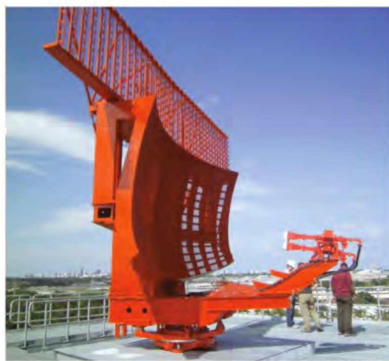
The ASR-9 is a typical air traffic control radar with both PSR (bottom) and SSR (top) antennae
