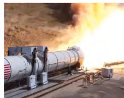
A ground-based test of one of the Space Launch System's SRBs
