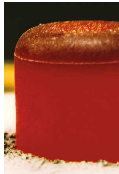
The heat from this glowing pellet of plutonium oxide can power a spacecraft
