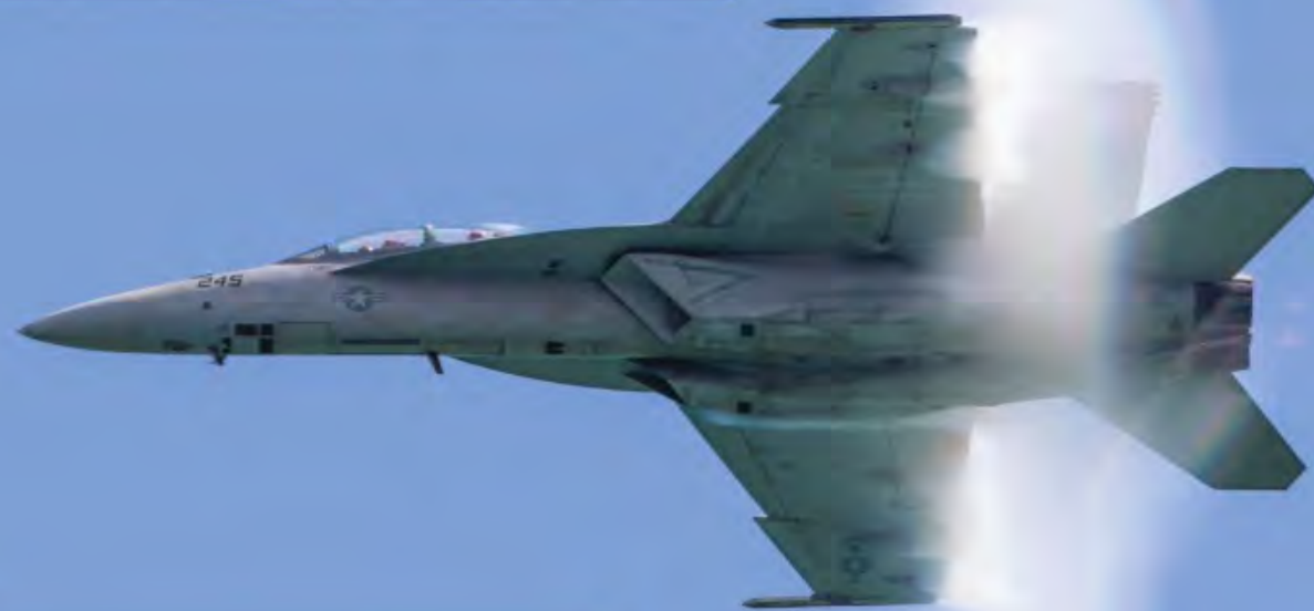
A shock wave and air molecules form a cloud around the midsection of a F/A-18E/F Super Hornet as it approaches the speed of sound
