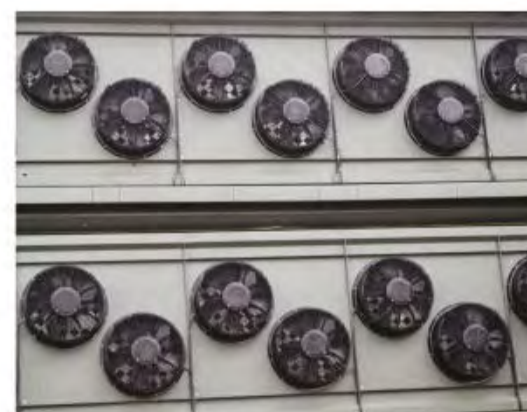
Climeworks uses direct air capture, drawing in air with large fans
