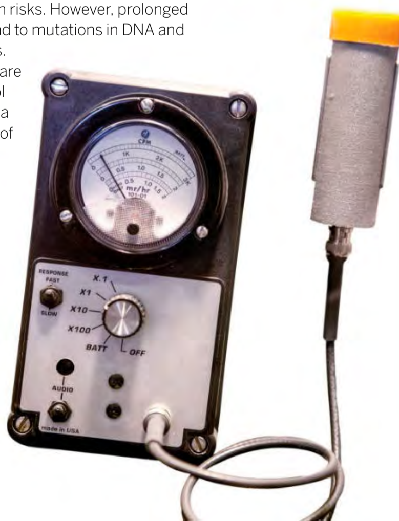
A Geiger–Müller counter used in detecting radioactivity and radiation
