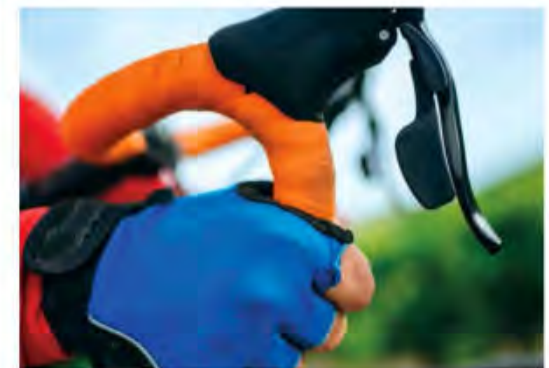
To change gears, a cyclist reaches for the lever in front of the handlebars
