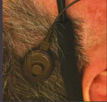
The Argus implant's camera and transmitter signal to the optic nerve
