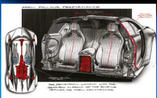
The cabin design is constrained by having the gearbox in front of the engine
