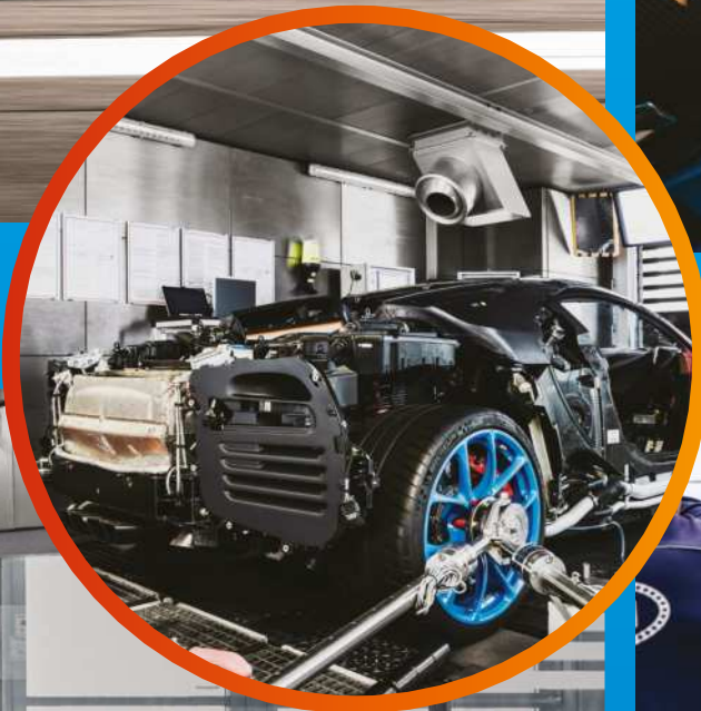
The rolling dynamometer is so powerful that excess electricity is fed to Molsheim's grid
