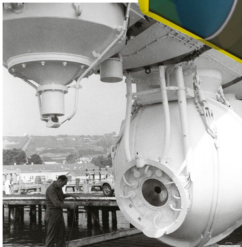
A close-up view of the Trieste's pressure sphere, clearly showing the Plexiglas observation window and instrument leads
