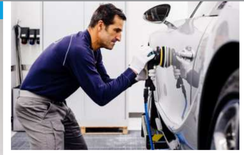
Several days can be spent smoothing out imperfections before paint is applied to the bodywork
