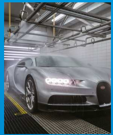
The Chiron is drenched by monsoon-strength showers to check for leaks
