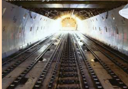
The cargo bay of a freight airliner, including a conveyer belt for hauling goods
