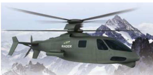
The Raider's cockpit can fit two pilots and the cabin will have space for six soldiers
