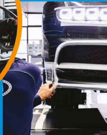
Plastic foil coats the Chiron during its test-drive so the paintwork isn't chipped
