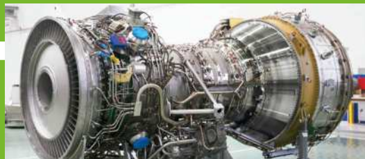
The 6.5-tonne turbine is paired with electric motors and diesel generators
