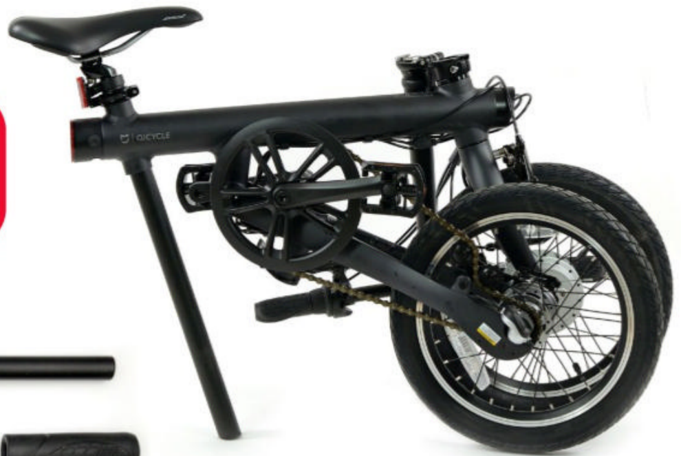
When folded, the wheels come together and the handlebars fold downwards
