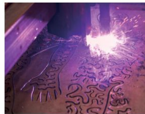
This detailed metal sculpture is being cut using a plasma cutter
