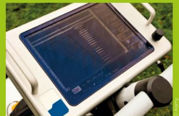
Ground-penetrating radars are used to detect irregularities underground
