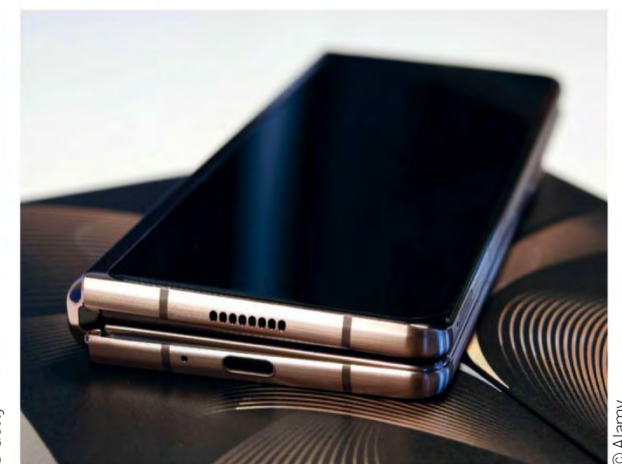
Small bristles in the gap along the phone's spine help to repel dust
