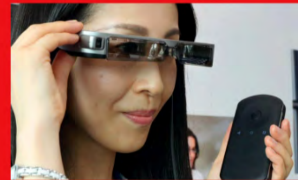
The Epson Moverio BT-300 connects to a trackpad to control a drone
