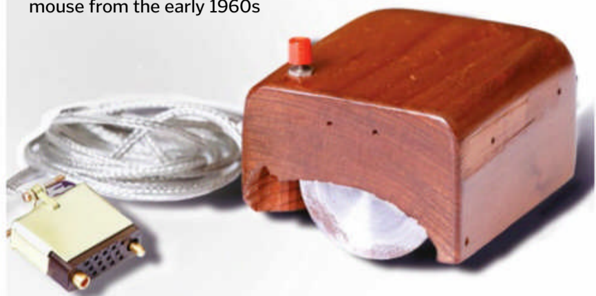
The prototype Stanford Research Institute (SRI) mouse from the early 1960s
