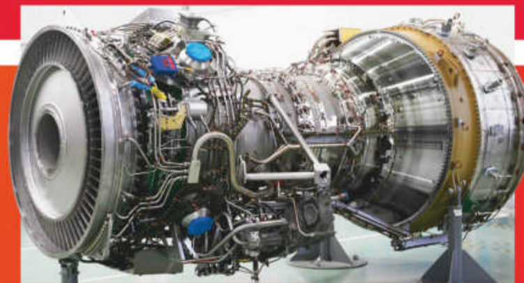
The 6.5-tonne turbine is paired with electric motors and diesel generators
