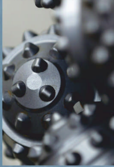
This grinding drill bit can bore through 7,500 metres of rock and mud below the ocean floor
