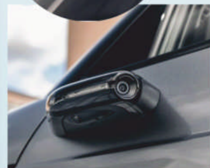
The mirrors stick out for a wide view, but have a flat shape to remain aerodynamic
