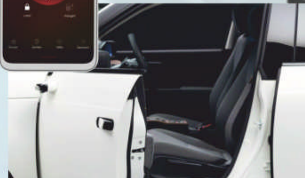
When the key fob is close, the car picks this up and the door handle pops out as the door unlocks
