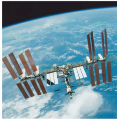
The International Space Station uses electrical power from 262,400 solar cells
