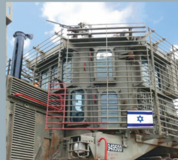
The cage armour around the cabin shields against rocket-propelled grenades
