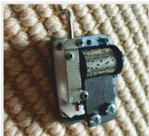
The pins on the metal cylinder pluck the prongs below
