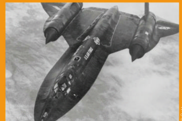
The Lockheed Blackbird SR-71 was a stealth aircraft built with lightweight titanium alloys
