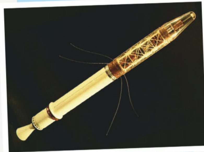
Explorer 1 was the first spacecraft to detect the Van Allen radiation belt around the Earth
