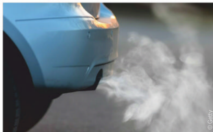
The product of a car's combustion engine is around 13% carbon dioxide, 13% water and 73% nitrogen
