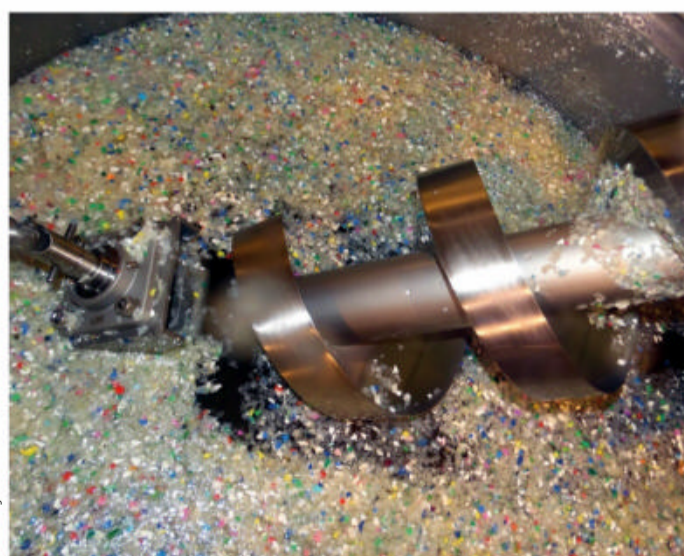
Plastic waste is shredded into pellets before impurities such as paper labels are separated
