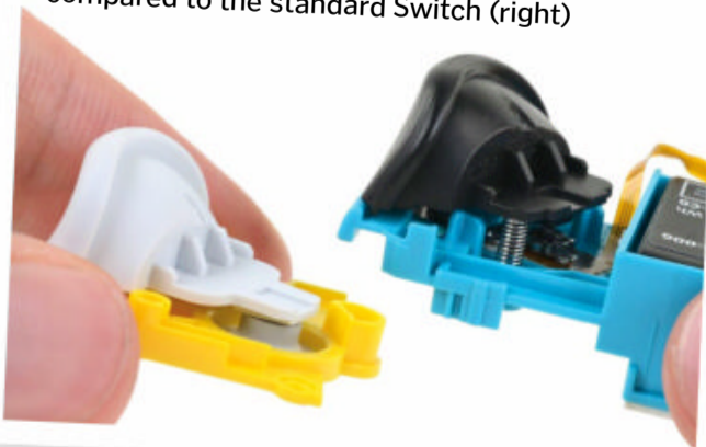
The Switch Lite's updated shoulder button (left), compared to the standard Switch (right)
