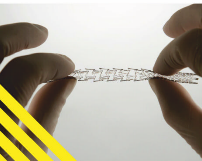
Nitinol wire has the ability to 'remember' its shape when placed in hot water
