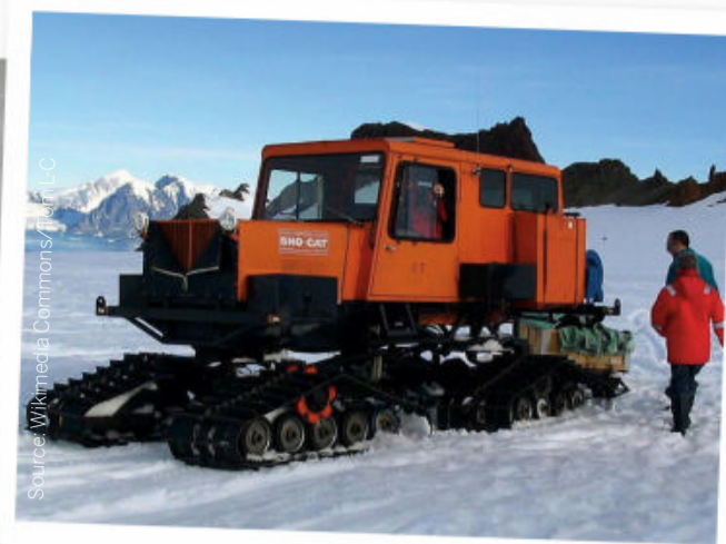
This Sno-Cat shows how belts rather than tyres spread weight more evenly on snowy surfaces
