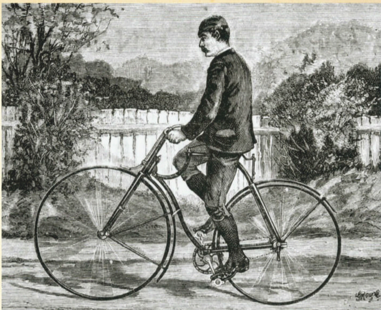
The Rover safety bicycle was far safer and more stable than previous bikes and formed the blueprint for future designs
