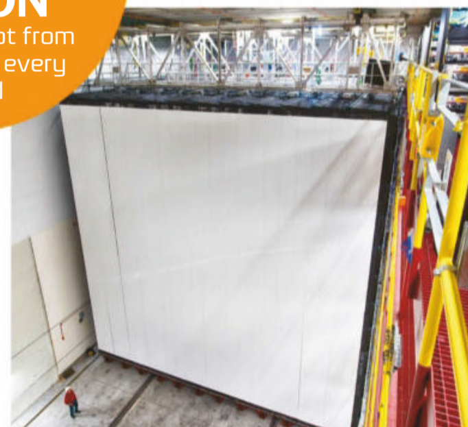
The NOvA far detector is the biggest free-standing plastic object in the world
