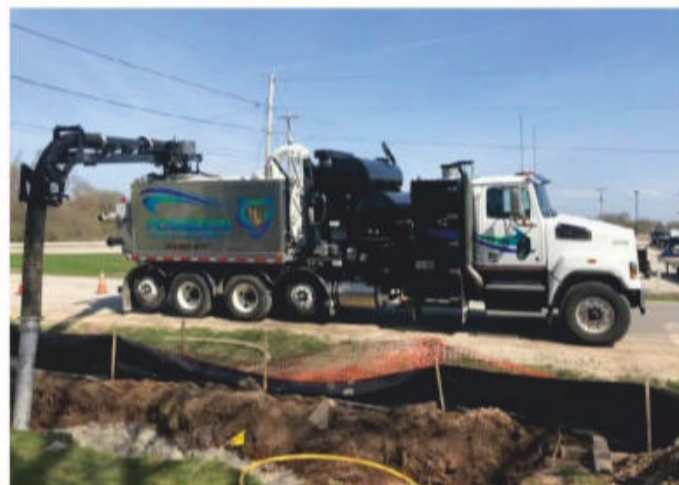
Hydrovacs are used to access underground infrastructure, including cleaning US storm drains
