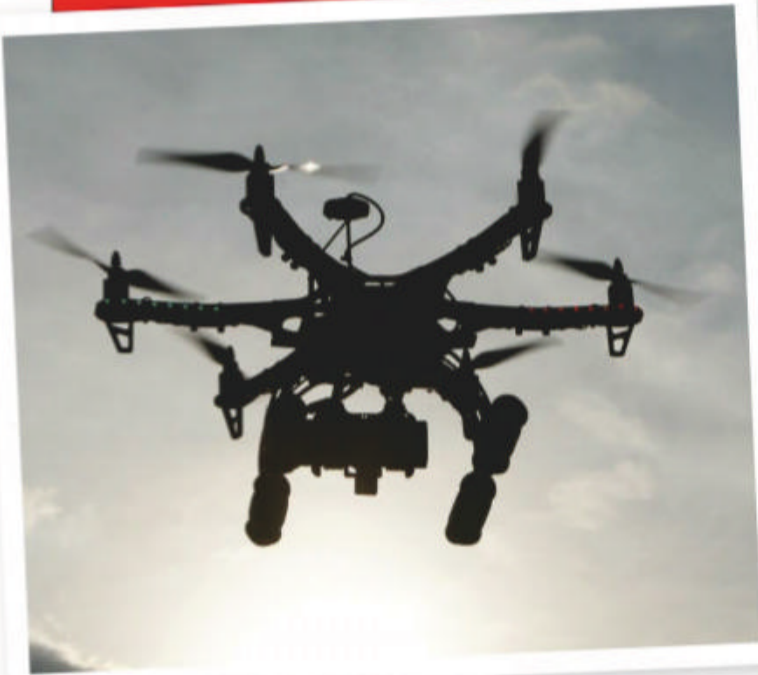
LiDAR systems and digital cameras are attached to drones to document inaccessible sites
