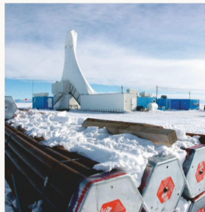
Drill rods await use just outside the ANDRILL facility in Antarctica
