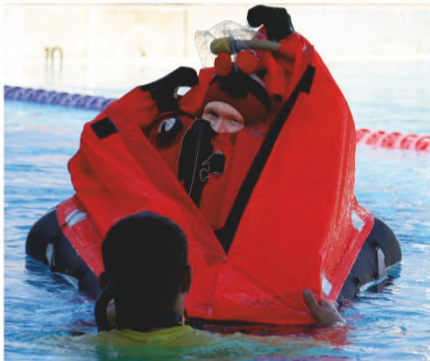
Submariners can escape sunken submarines wearing inflatable escape suits that also act as life rafts
