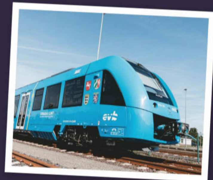
The Coradia iLint is completely emission-free, powered only by hydrogen and oxygen
