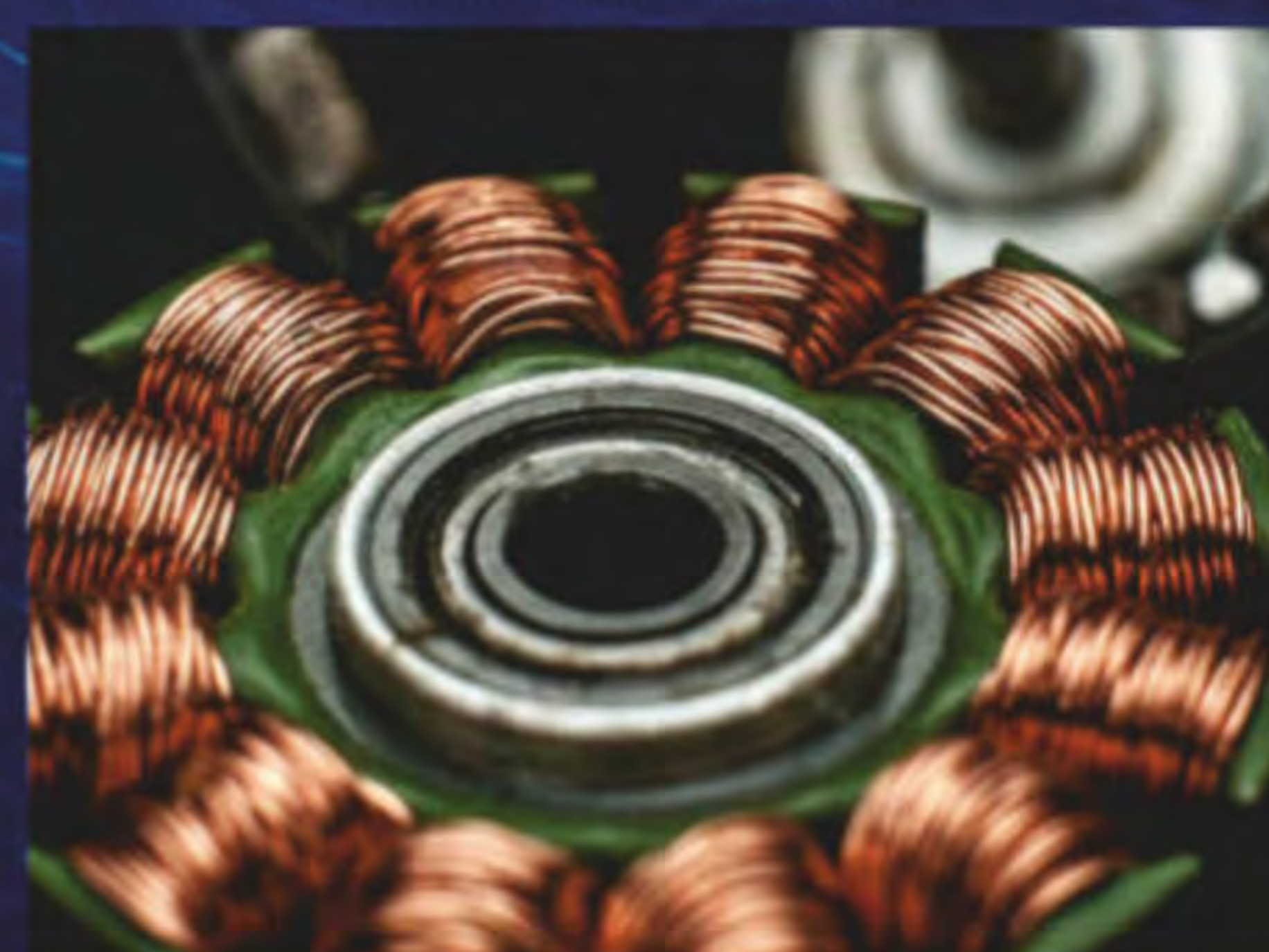
Coils of copper wire generate magnetic fields that make this electric motor spin
