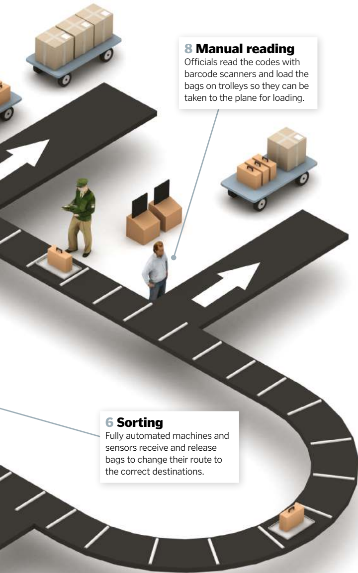
Barcodes on the luggage tag, tray and chassis are registered together to send the suitcase on its journey
