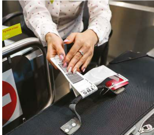
Barcodes on the luggage tag, tray and chassis are registered together to send the suitcase on its journey
