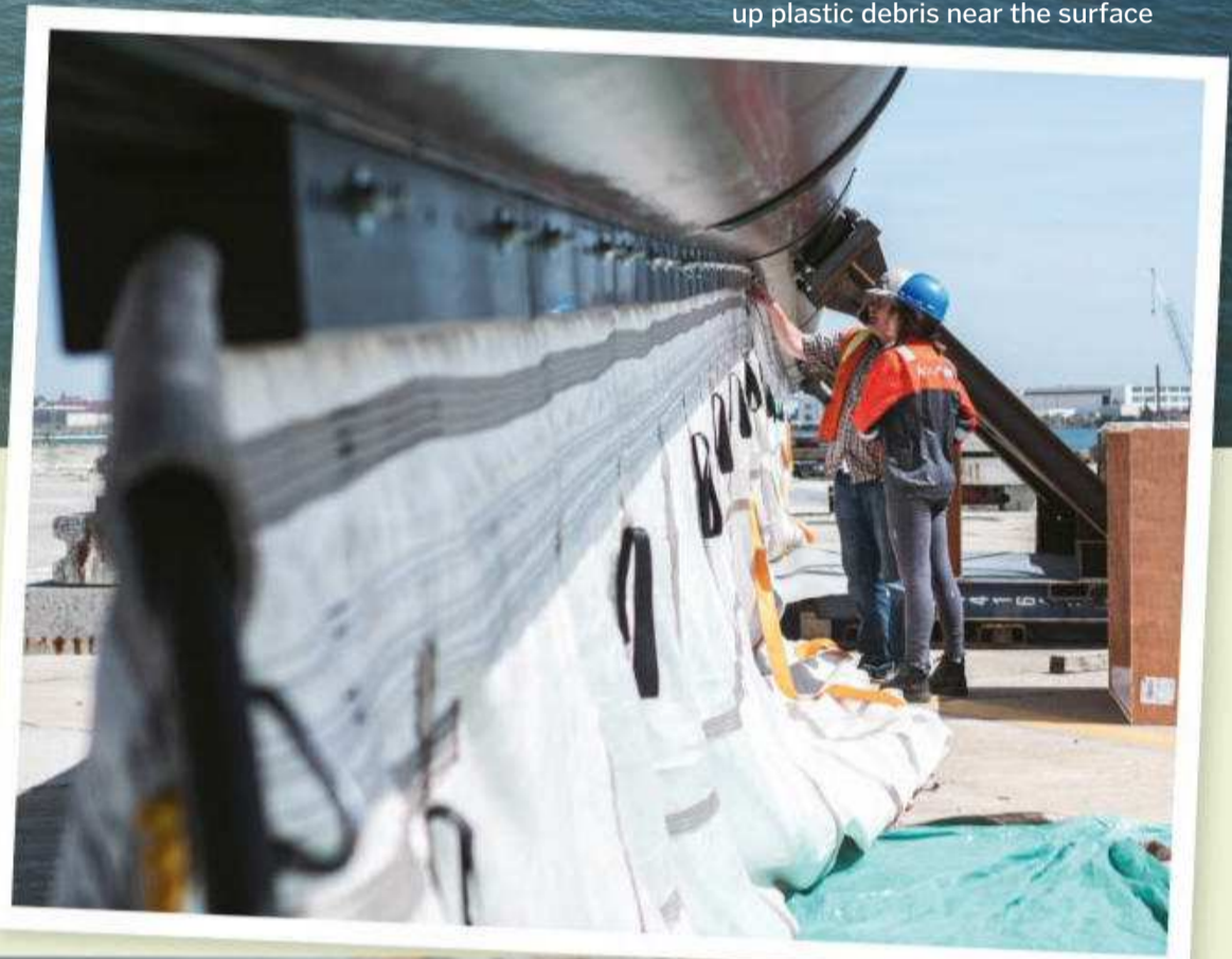
The skirt (pictured below) will extend beneath the float to sweep up plastic debris near the surface
