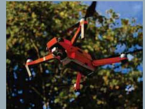
KSAR's DJI's Mavic drones can cover a range of over 10km, providing high-resolution real-time video
