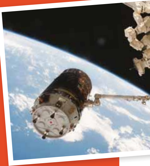
An HTV cargo spacecraft being grabbed by a robotic arm during docking on the ISS
