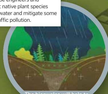
The bioswales will help to control and clean the highway's water runoff during rainstorms
