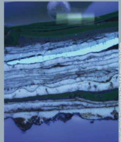
Zinc layers in a paint cross-section will glow under UV light
