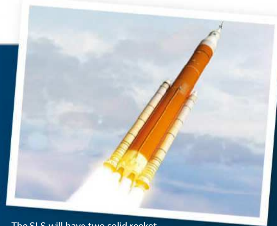
The SLS will have two solid rocket boosters on the side and will not be reusable
