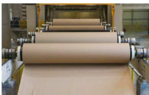
Above: Paper is pulled through a series of cylinders during the process to help dry and smooth the product
