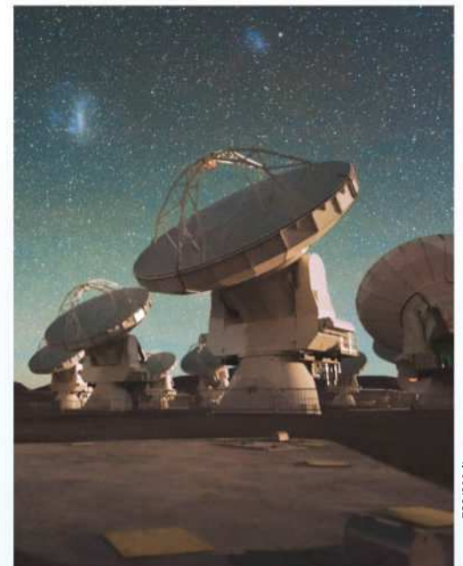
The ALMA telescope is made up of 66 antennas, and is used to study light from some of the coldest objects in the universe
