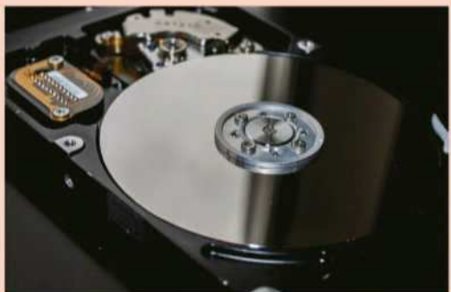
The disc (called a platter) within your hard drive stores information in binary form, and the arm mechanism with a read/write head moves across it to read or store data
