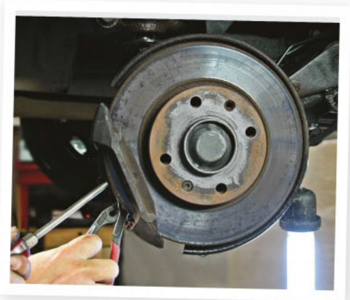
Regular friction causes the brake discs and pads to wear over time, meaning that they need to be replaced frequently
