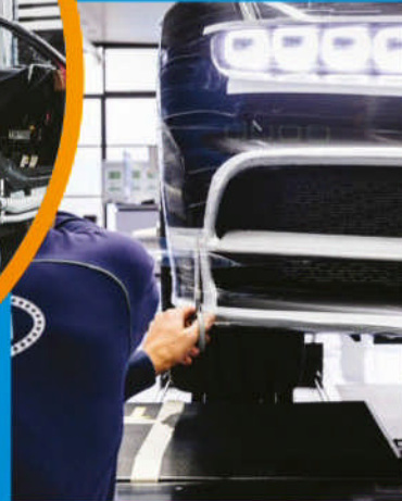
Plastic foil coats the Chiron during its test-drive so the paintwork isn't chipped
