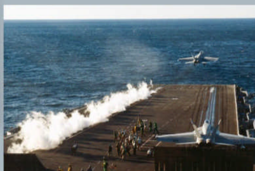
On land it can take 1,500 metres to get a fighter jet airborne, but with the steam catapult it takes only 100 metres
