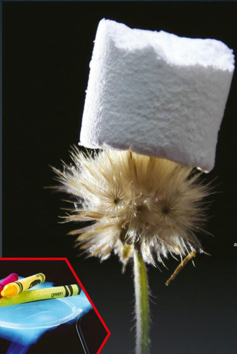
This amazing feat is possible thanks to the aerogel's thermal insulation properties
