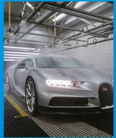
The Chiron is drenched by monsoon-strength showers to check for leaks
