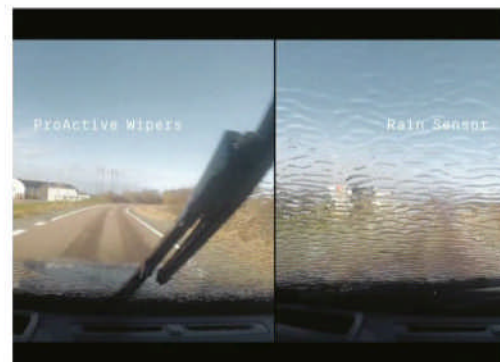
Activated before the windscreen is drenched, PAW minimises the time the driver's view is impaired
