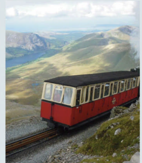
Mountain railways sometimes use a racked rail and cogwheel train for better grip
