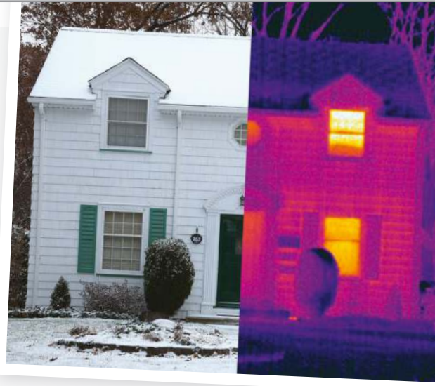
Thermograms detect infrared radiation and can help identify areas where the most heat is lost (shown in yellow and orange)
