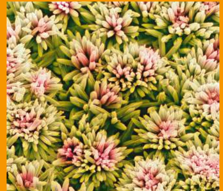
A scanning electron microscope image showing crystals of limescale inside a kettle
