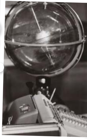
A celestial training device was a globe within a globe that showed the key coordinates for navigation in Earth's orbit
