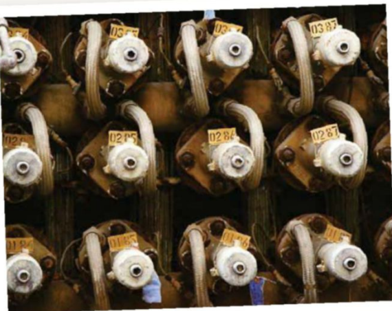
Close up of the tubes that fed uranium into the Hanford reactor
