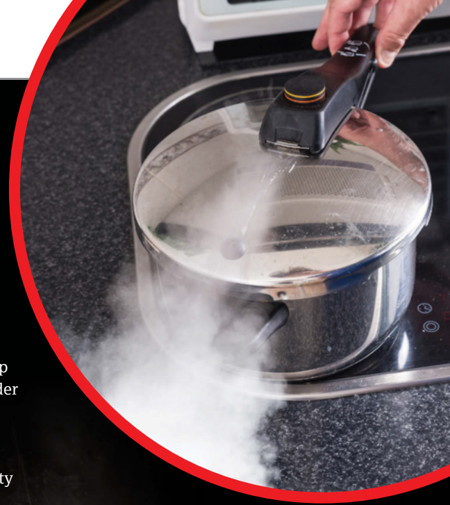
When the pressure gets too high, a valve on the lid releases some steam
