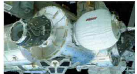
The inflatable module is composed of an aluminium structure, layers of fabric and an internal bladder system
