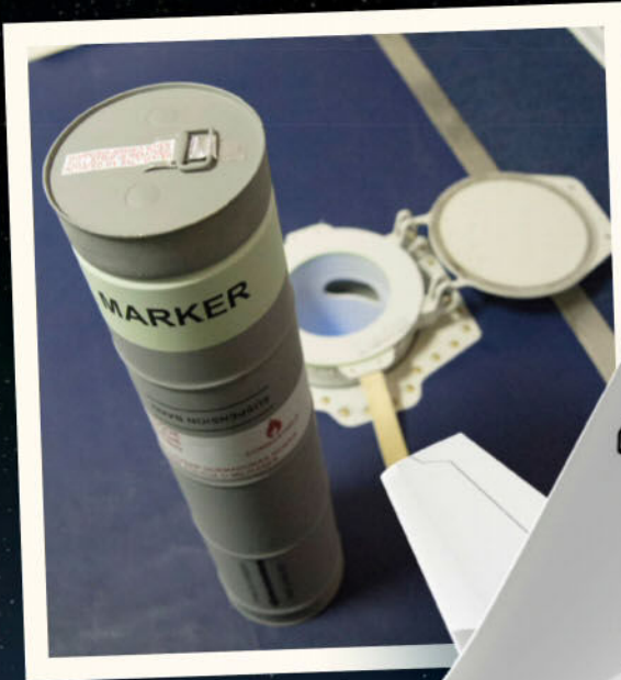
Sonobuoys listen for sounds in the water and relay information to the aircraft
