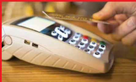
Some contactless payment cards use RFID technology to send information wirelessly to the card reader
