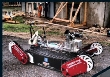
The Quince's unique wheel mounts let it both roll and step over uneven surfaces
