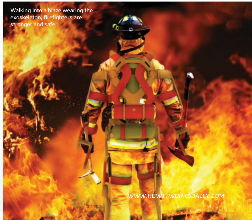
The exoskeleton is built to carry specialised kit, including water guns and rescue tools
