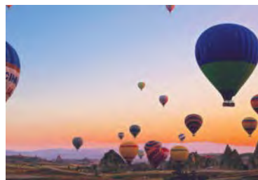
Hot air balloons float because the hot air inside the envelope weighs less than the same volume of cold air outside
